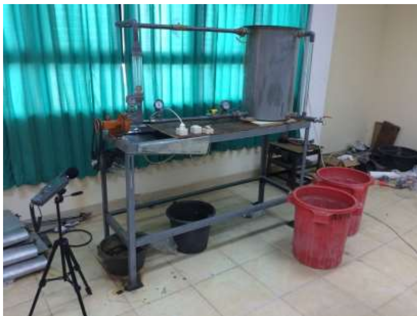
Gambar.10 Detail instalasi instrument penelitian pompa sentrifugal
